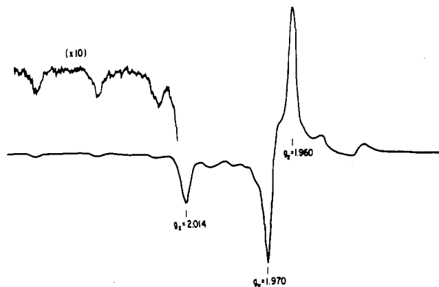
Figure 5. Frozen-solution spectrum of [\text{MoOL}]^+ , taken on a Varian E-4 spectrometer with the following parameters: scan range 400 G, field setting 3400 G, time constant 1 s, scan time 8 min, modulation amplitude 0.63 G, modulation frequency 100 kHz, power 5 mW, microwave frequency 9.472 GHz.
